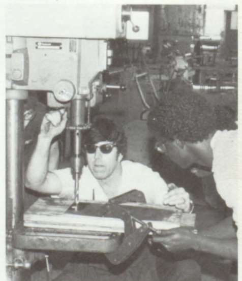
Mr. Sanders demonstrates to two of his students how to drill a hole in a steel plate.
