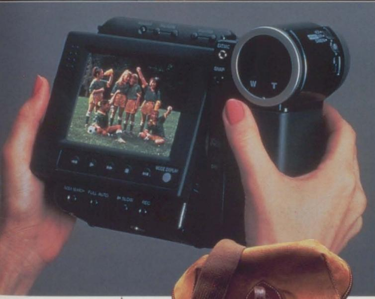
The point-and-shoot camcorder arrives with Sony's new Viewcam, in Hi-8 format with stereo sound, 4-inch color LCD screen, image stabilization, still and strobe effects. Viewcam and the even smaller Handycam allow you to film without lifting the camera to the eye.
