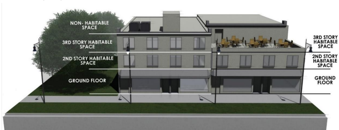
Figure 5.1.1. Building Height Illustrations
