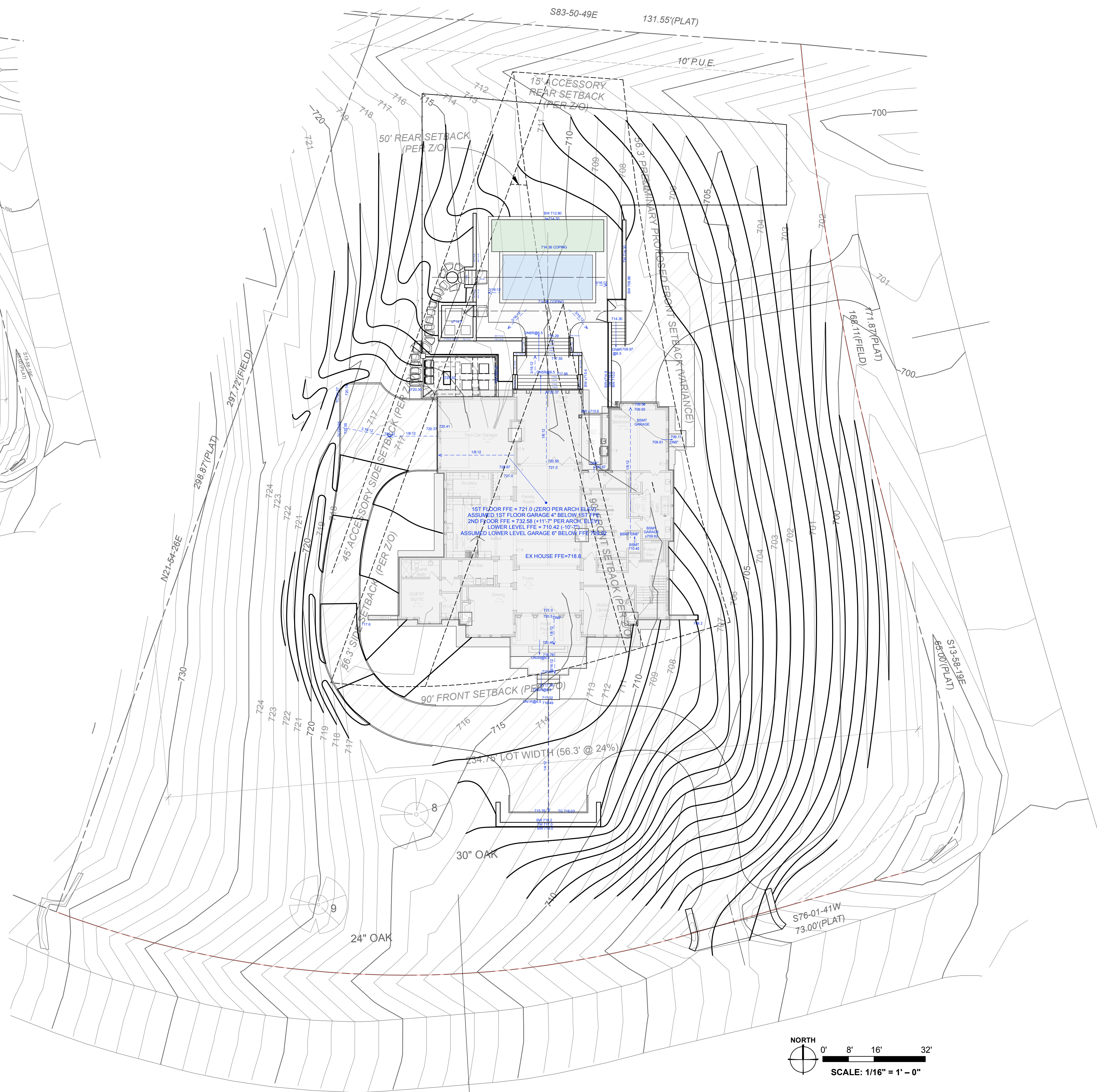
DETAIL 1: CONCEPT FINISH GRADE DIAGRAM/PLAN SCALE: 1/16" = 1'-0"
