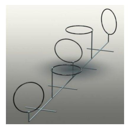
Teams are required to traverse each of five 46 cm rings, surface and return through the five rings. All Rings must be traversed in both directions. Fastest elapsed time wins. If a diver assist is required to move, untangle, etc. the ROV an additional two minutes will be added to the time. Teams will have two attempts at the course during their 15-minute time allocation. See Obstacle Course Scoring sheet for more details.
