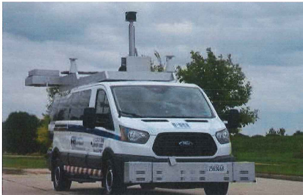
ERI's Automated Pavement Data Collection Vehicle System
