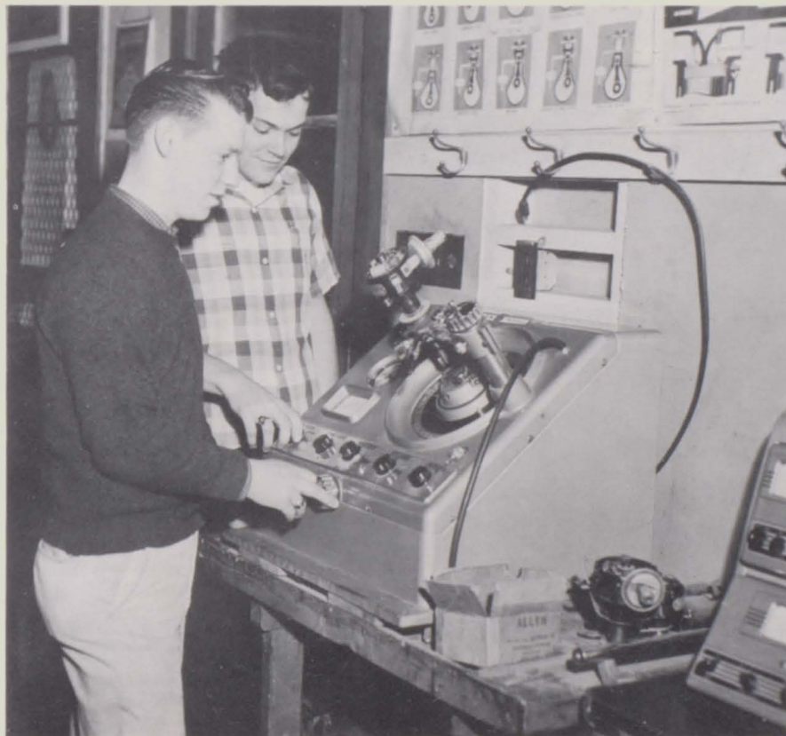
David Costain and Allen Baker test a set of points on the syncrograph.
